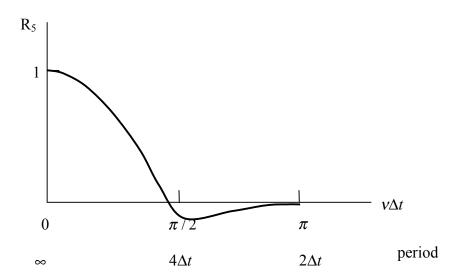
A perfect "low pass filter" would have a response equal to 1 for low frequencies lower than a critical frequency  $V_c$ , and zero for higher frequencies:
