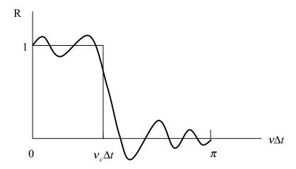
For this reason, Lanczos introduced a different "ideal" filter (the Lanczos filter), that instead of a step function, has a ramp around the critical frequency, with a width that depends on the number of terms L of the filter:
