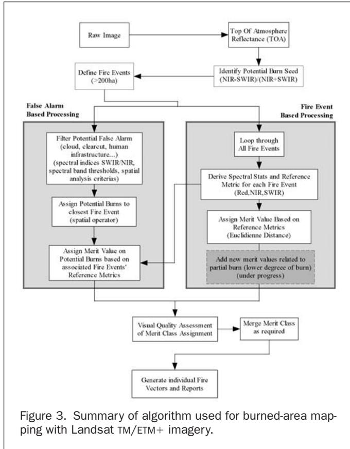
Figure 3. Summary of algorithm used for burned-area mapping with Landsat TM/ETM+ imagery.
