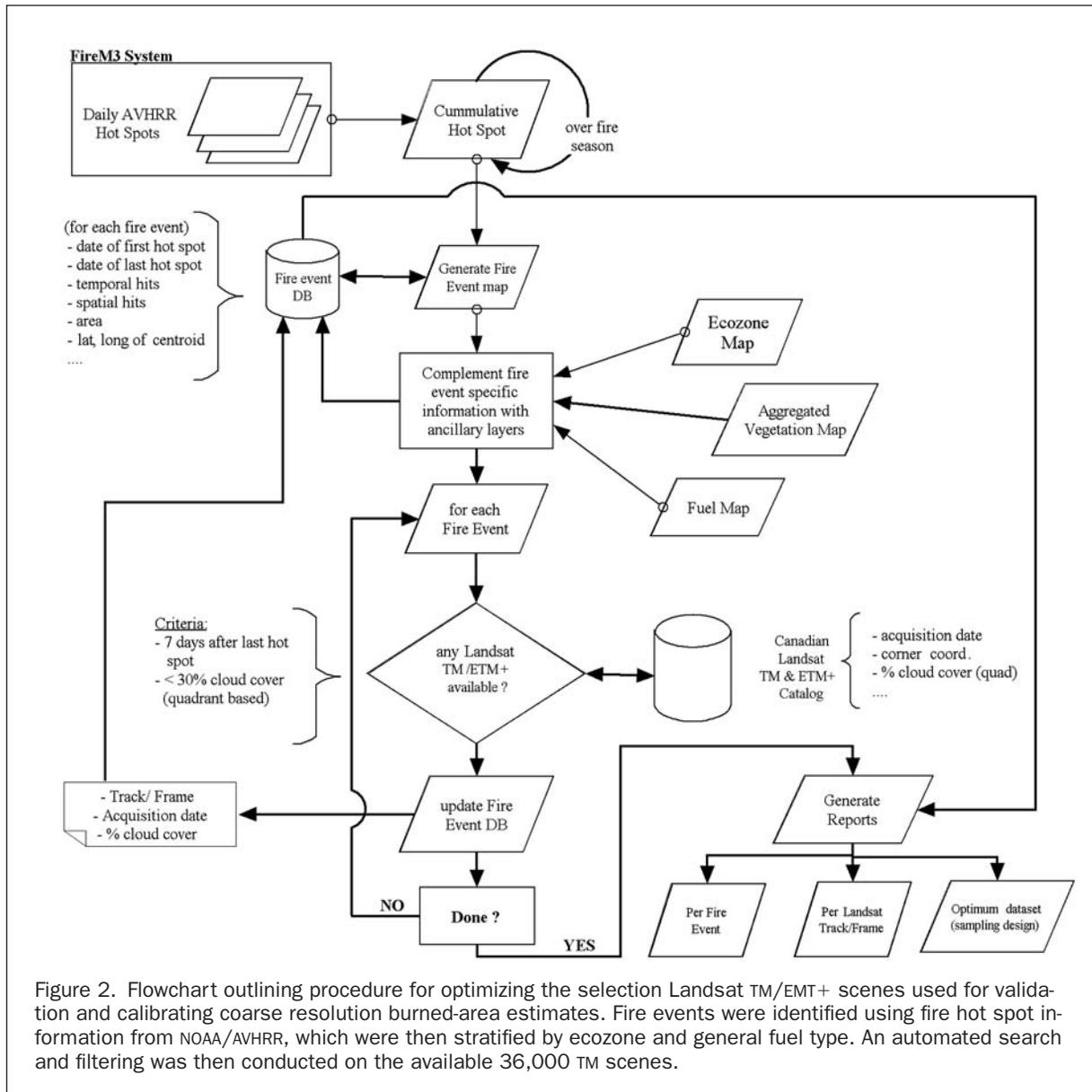
Figure 2. Flowchart outlining procedure for optimizing the selection Landsat TM/ETM+ scenes used for validation and calibrating coarse resolution burned-area estimates. Fire events were identified using fire hot spot information from NOAA/AVHRR, which were then stratified by ecozone and general fuel type. An automated search and filtering was then conducted on the available 36,000 TM scenes.
