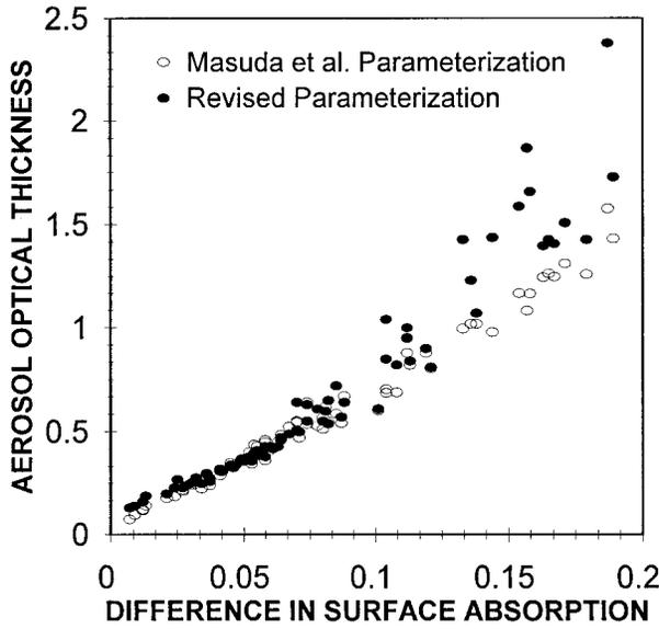
FIG. 8. Comparison of the aerosol optical thickness as a function of the difference in normalized surface absorbed flux derived from the two parameterization schemes using all data under study.
