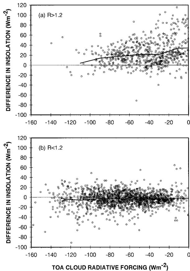
FIG. 5. Same as Fig. 4 but the data are grouped according the ratio of cloud radiative forcing ( $R$ ) (a) greater and (b) less than 1.2. Also plotted are the curves of the mean differences in insolation computed for each  $CRF_{TOA}$  bin of  $20 \text{ W m}^{-2}$ .
