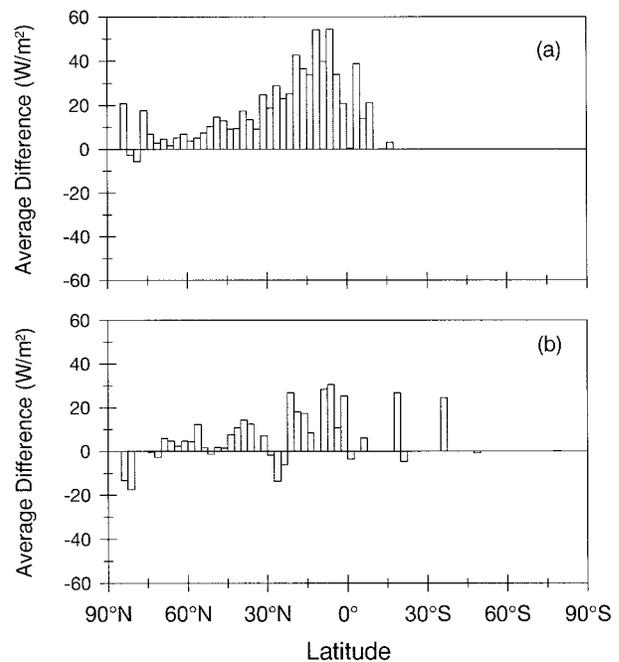
FIG. 2. Zonal comparisons of the monthly mean SSRB estimated from ISCCP using the algorithms of (a) Pinker and Laszlo (1992) and (b) Rossow and Zhang (1995) against ground-based observations from GEBA.
