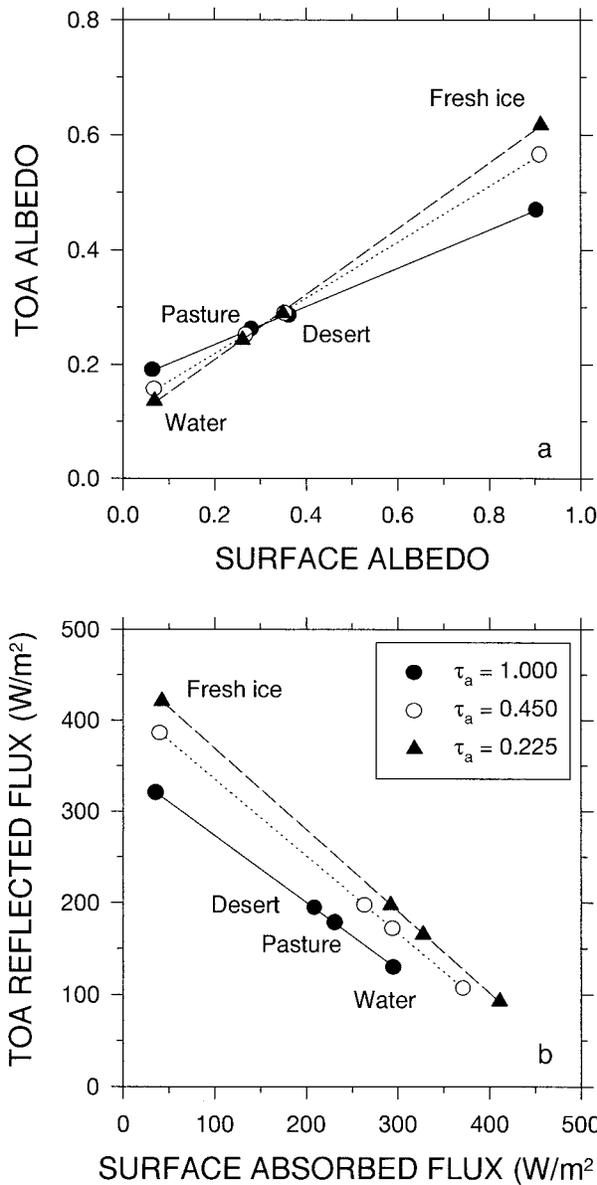
FIG. 3. Sensitivity tests of the relationship (a) between TOA and surface albedos and (b) between TOA reflected flux and surface absorbed flux for varying aerosol optical thickness. The data were simulated using a radiative transfer model with the continental aerosol under clear skies over different types of surfaces.
