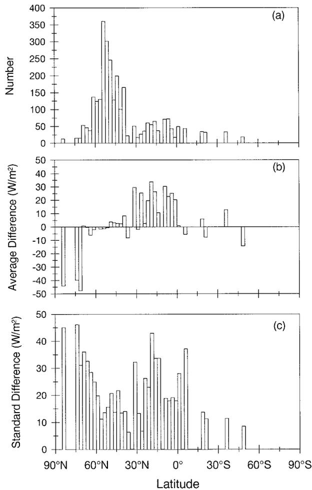
FIG. 1. Zonal comparisons of the monthly mean SSRB estimated from ERBE (Li and Leighton 1993) against ground-based measurements archived in GEBA: (a) number of data samples in each  $2.5^\circ$  latitude zone, (b) mean difference (satellite minus surface), and (c) standard difference.
