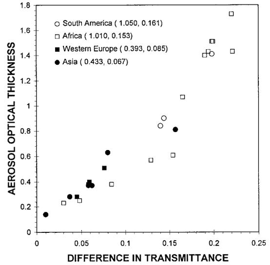
FIG. 9. Estimated aerosol optical thickness as a function of the atmospheric transmittance derived from the new parameterization for heavy smoky or polluted conditions as identified in Fig. 6 (original  $R > 1.2$ ) over four regions.
