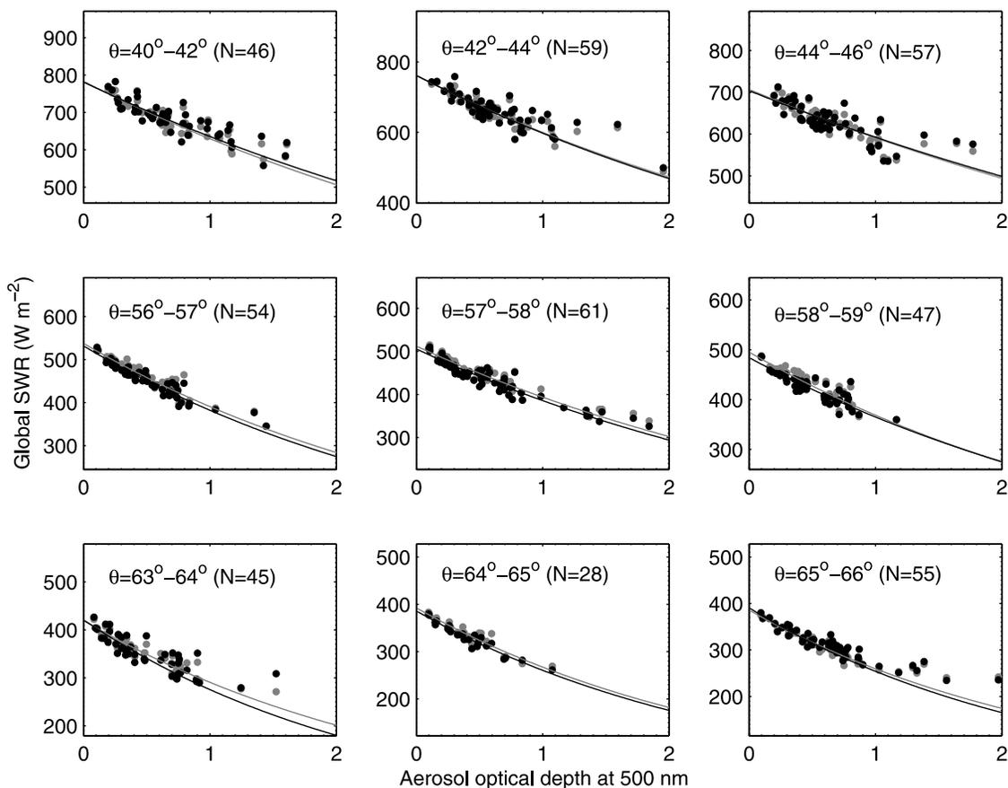
**Figure 7.** Scatterplots of global shortwave irradiance as a function of the aerosol optical depth at 500 nm for nine solar zenith angles. Measurements and model simulations are represented by shaded and solid dots, respectively. The shaded and solid curves represent the fitting results using an exponential equation to the measurement and model simulation, respectively.
