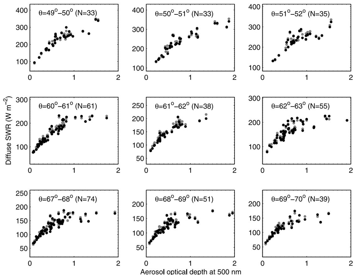
**Figure 11.** Scatterplots of diffuse shortwave irradiance as a function of the aerosol optical depth at 500 nm for nine solar zenith angles. Measurements and model simulations are represented by shaded and solid dots, respectively.
