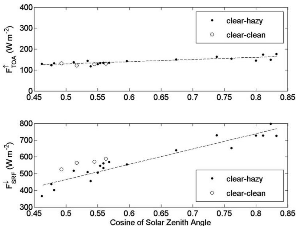
**Figure 13.** Solar irradiance (top) reflected at the top of the atmosphere from the CERES SSF product and (bottom) incoming on the ground measured on the ground for clear-clean ( $\text{AOD} < 0.2$ ) and clear-hazy conditions ( $\text{AOD} > 0.2$ ) at Taihu. Data are from September to December 2005.
