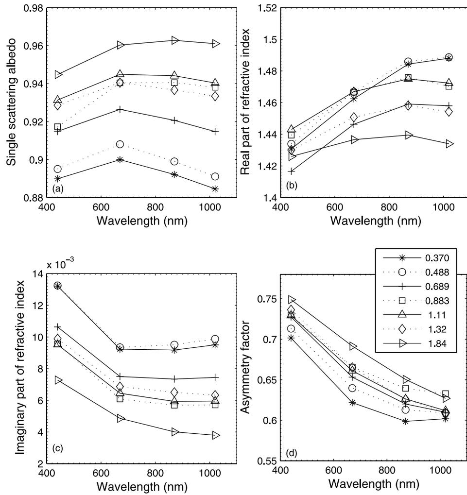
**Figure 3.** (a) Averaged aerosol single scattering albedo, (b) real part of refractive index, (c) imaginary part of refractive index and (d) asymmetry factor in each of the seven bins of aerosol optical depth at 500 nm, which is calculated if more than 10 almucantar scans are available.
