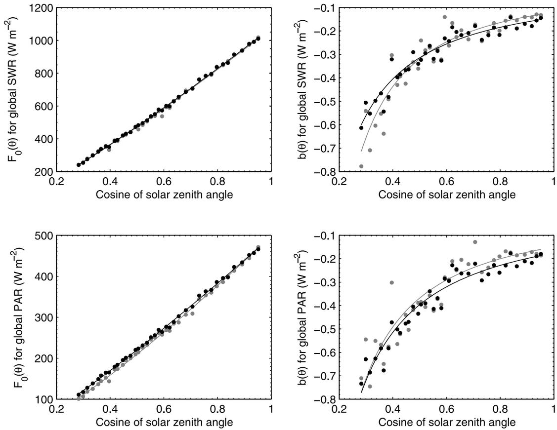
**Figure 8.** Scatterplots of parameters  $F_0(\theta)$  and  $b(\theta)$  as a function of the cosine of the solar zenith angle for (top) global shortwave irradiance and (bottom) global PAR.
