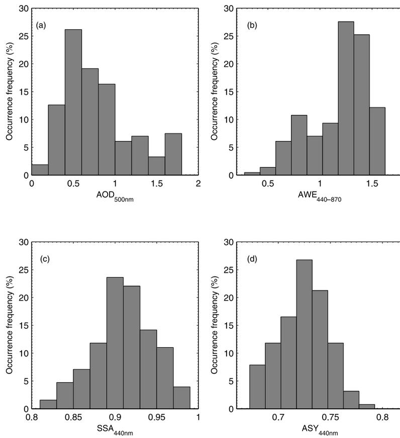
**Figure 1.** Histograms of (a) aerosol optical depth at 500 nm, (b) Ångström wavelength exponent, (c) single scattering albedo at 440 nm and (d) asymmetry factor at 440 nm.
