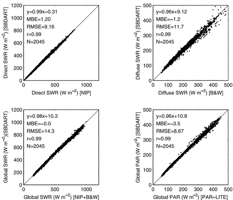
**Figure 6.** Comparisons between the model simulations and the observations of (top left) direct, (top right) diffuse, (bottom left) global, and (bottom right) PAR radiation (unit is W m<sup>-2</sup>).
