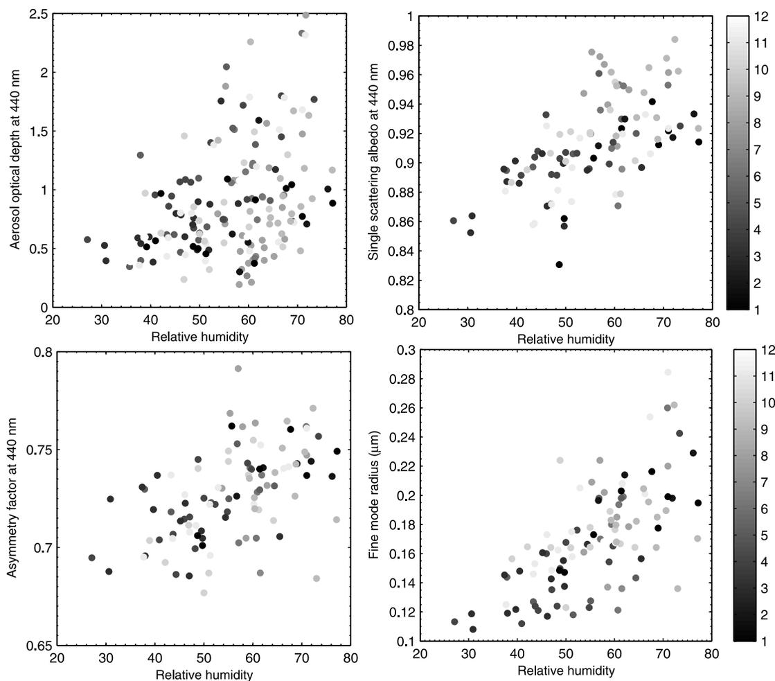
**Figure 5.** Relationships between relative humidity and the aerosol optical depth, single scattering albedo, asymmetry factor and fine mode radius for data from September 2005 to August 2006. The data points in each month are represented by different shading.
