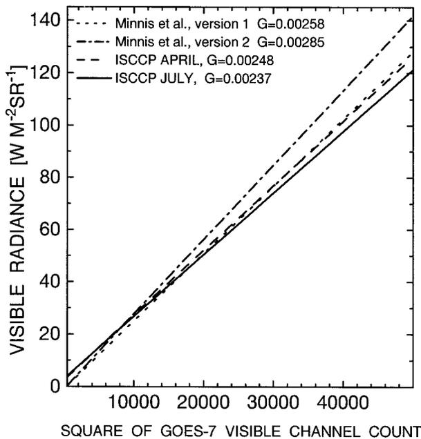
FIG. 3. A comparison of ISCCP and NASA LaRC calibration for *GOES-7* VISSR visible channel. Plotted are the gains ( $G$ ;  $W m^{-2} sr^{-1}$ ) used in two versions of the *GOES-7* data generated by Minnis et al. (1995) and two months used in ISCCP.
