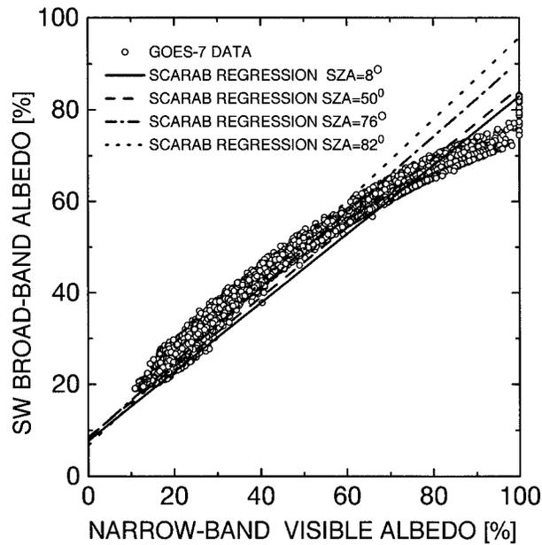
FIG. 14. Comparison of the relationship between narrow- and broadband albedos used for *GOES-7* and derived from ScaRaB measurements. Open circles denote broadband albedos derived from *GOES-7* algorithm adjusted to ScaRaB visible band using Eq. (2). The lines represent regressions obtained from ScaRaB, as given by Eq. (3), for various values of the SZA.
