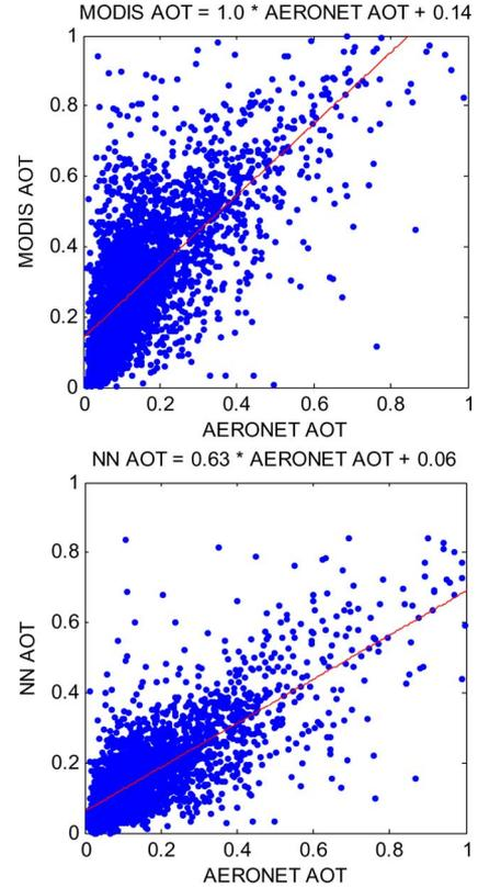
Fig. 1. (a) AERONET AOT versus MODIS AOT. (b) AERONET AOT versus neural network retrieval.
